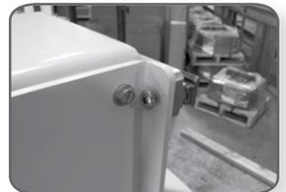
Ensure that the seat support is level and tighten the two (2) front and two (2) rear leveling bolts.
