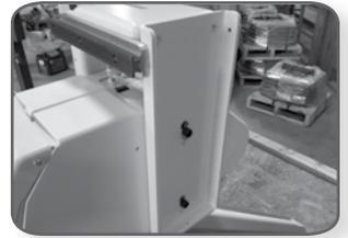
Secure the rear seat support to the footrest/seat support using the two (2) hex-head bolts and washers.
