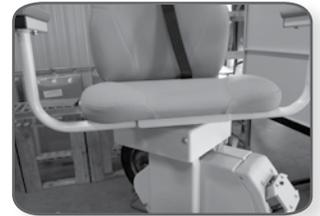
**Step 9:** Attach the swivel pin bracket with the flat side towards the footrest support using the two (2) hex head bolts and washers. Ensure that one of the swivel pins is engaged into the slot in the swivel cam.
