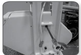
**Step 6:** Connect the footrest cable to the 6-pin connector on the chassis.
